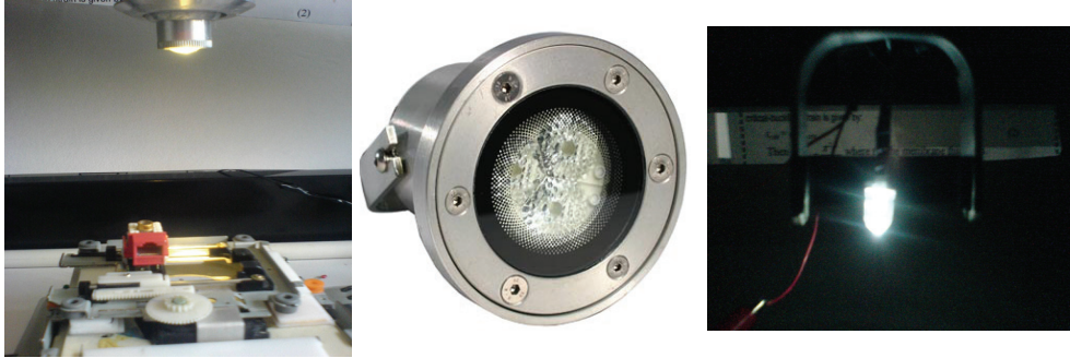
Fig. 18. (a) Dirigible X-lamp LED IL51, as a sample and the XY table. (b) Lamp IL/1 L3 (with a 3 LED array; and (c) single white LED
